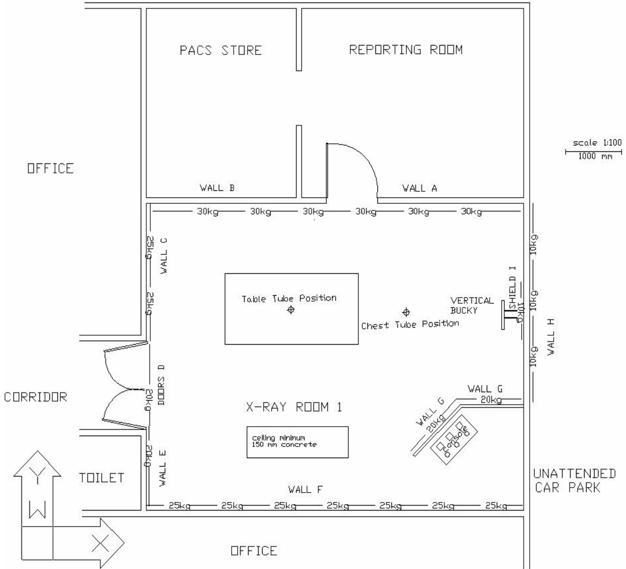
Figure 6: Sample shielding plan drawing
